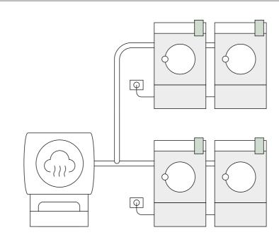
Thermal stability, great drying quality and easy machine management. We add to these innate characteristics of the steam system our special removable steel mesh filter, placed at the air inlet of the battery. So, protected from dust and lint, the battery remains clean and efficient for a long time (up to approximately 28 cycles) and you save time and effort.
